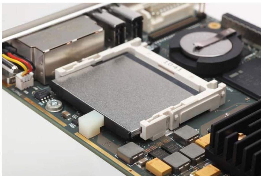
CFast™ Card Fixation w. Mounting Block
