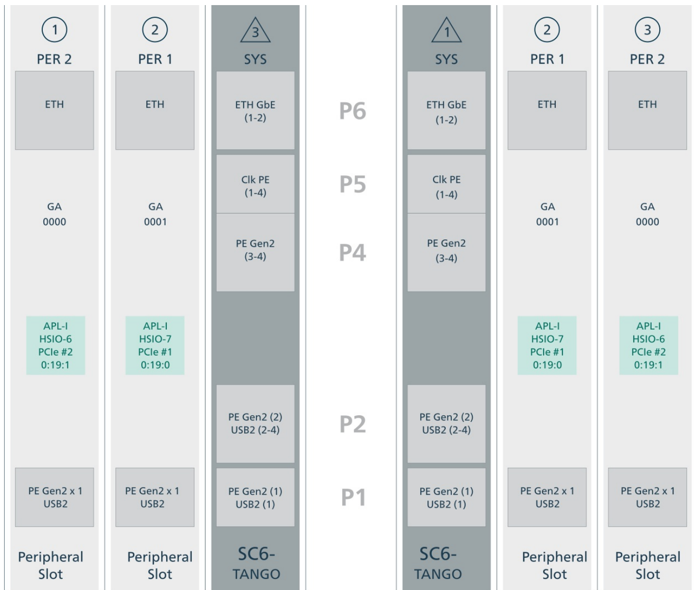
1+2 Slots backplane resources (system slot right) Peripheral slot target in brackets Pin assignment according to CPCI-5.0 specification
